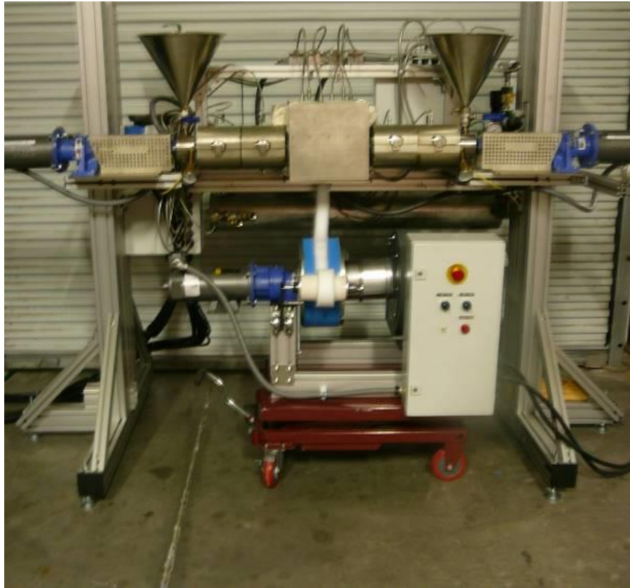
LBS-100 Meltblown arrangement with forming drum
