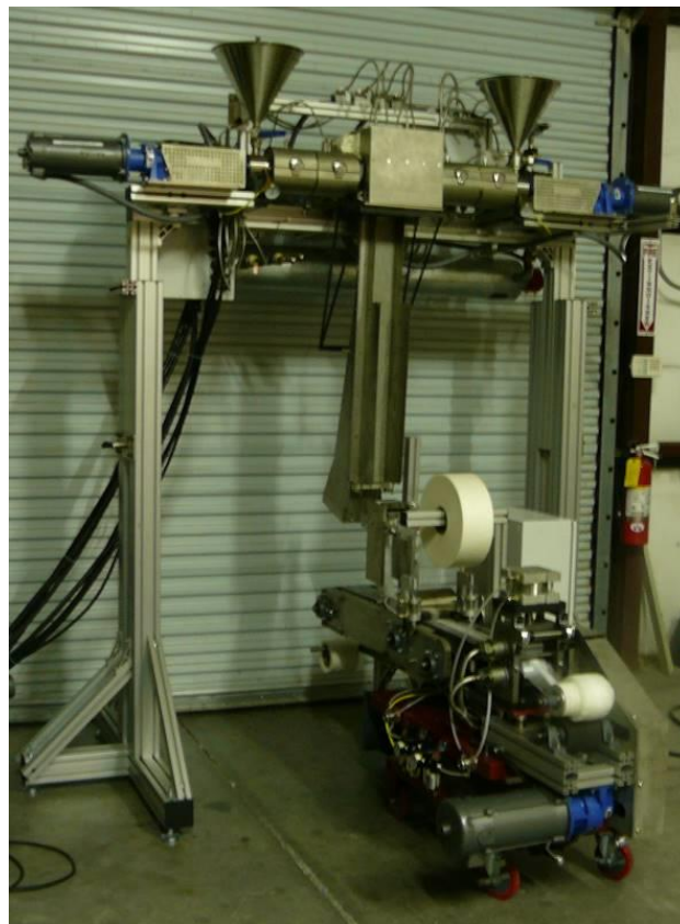
LBS-100 Spunbond arrangement with quench (air chiller & blower connection not shown), slot aspirator, web former w/ 2 sheet un-winds and, calender
