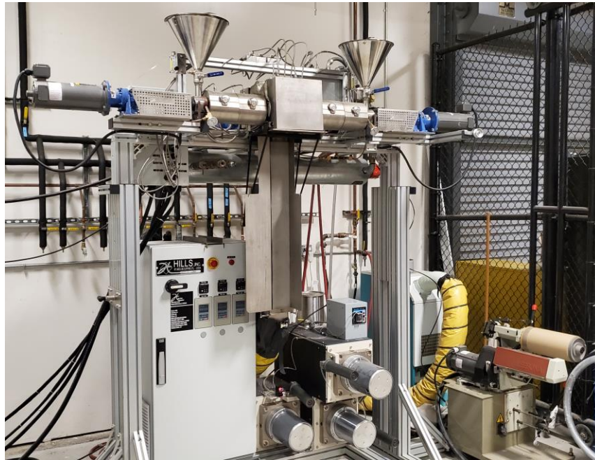
LBS-100 FDY fiber arrangement with 3 roll draw stand, metered spin finish, quench, self-contained air chiller, and 2000 m/m production winder
